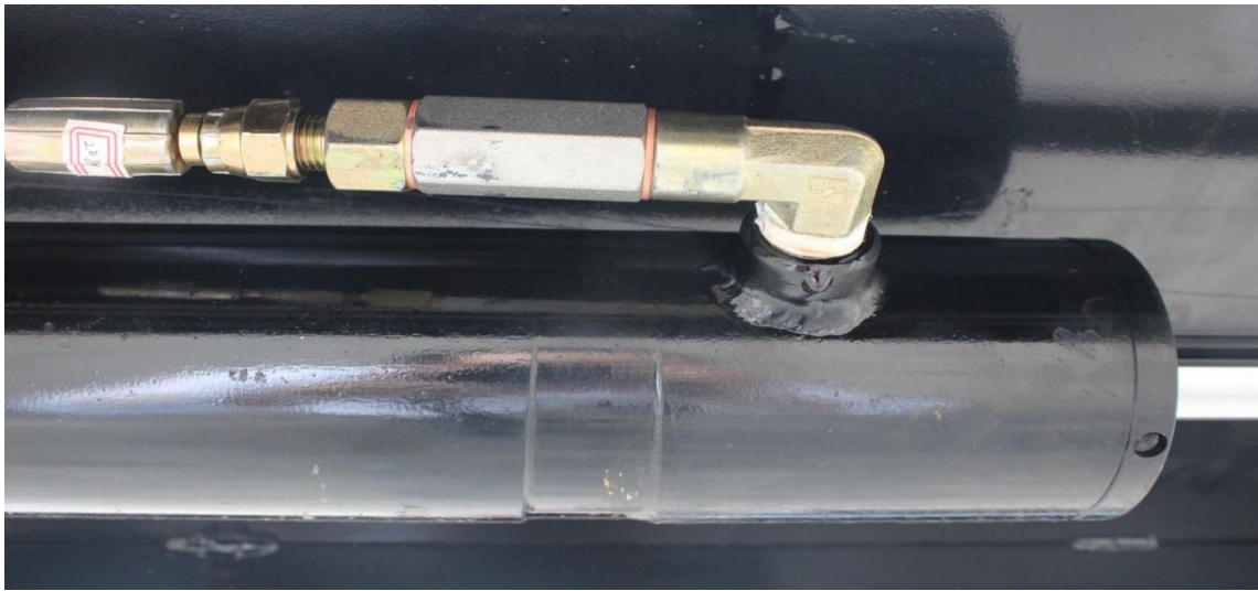
Hydraulic cylinder under the runway has explosion-proof valve
